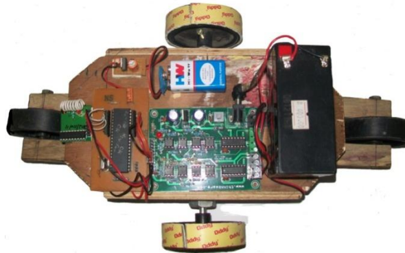
Fig. 7. Test vehicle of AGV and ultrasonic Instrumentation configuration
